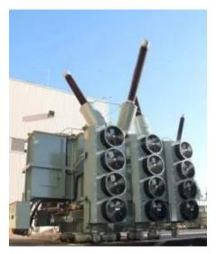
**Rugged and robust –** We design our OFAF transformer coolers to withstand vibration shock, seismic forces and thermal movement. Aluminium alloys are used as the standard for the tube, fin and tubeplate to minimise corrosion. We provide custom options as required. Components supporting the fans and cooler elements are protected to C3 as standard, increased to C5-M(H) when conditions dictate.
